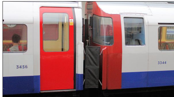
Figure 3-13 Between-car barrier installed on Transport for London.
