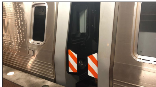
Figure 3-12 Between-car barrier installed on WMATA.
