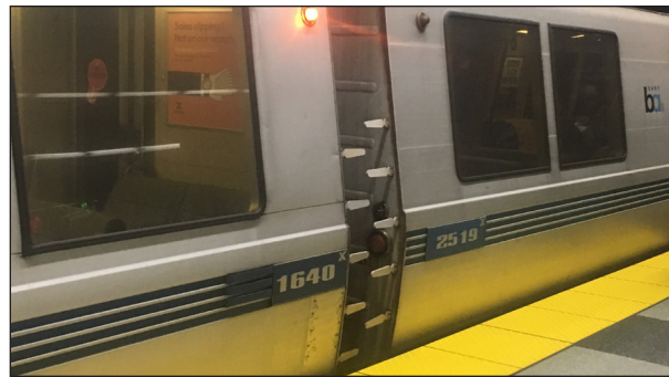
Figure 3-11 Between-car barrier installed on BART.
